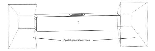
IMPORTANT: The areas marked need to be clear of obstacles in order for the stereo sound field to work effectively.
