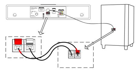
Note: The speaker wire is colour marked to make the job of identifying the correct wire for speaker terminal easy. Connect the wire marked with a red tab to the red terminal on the soundbar and the subwoofer.
