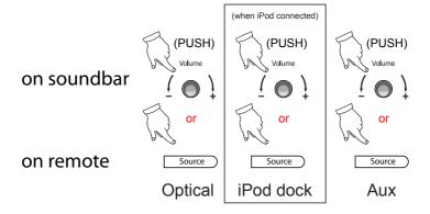
Source select: Press the 'Source' button on the remote (or briefly press the volume knob on the unit's rear) to cycle the sound source from optical, to analogue, to iPod dock. The iPod selection is skipped if no iPod is present (i.e. only 2 inputs are available when no iPod is in use).
