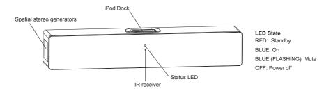
The orbitsoundbar produces most of the sound that you hear. It produces the main signal and stereo information. It also houses the amplifiers for itself and the subwoofer.
