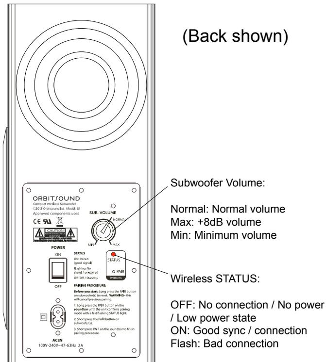
The subwoofer is a wireless active loudspeaker that produces powerful Hi-Fi bass. It has been designed specially to complement the soundbar.
