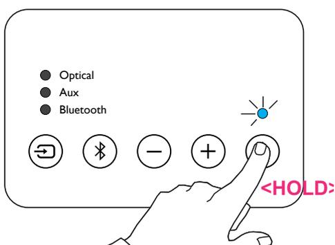
You may wish to reset the soundbar settings (returning everything to factory default). To do this, switch the unit on, then press and hold the power button for a few seconds on the control panel. The soundbar status light will flash, and then the soundbar will reset. Optical source will be selected when the reset is complete.
