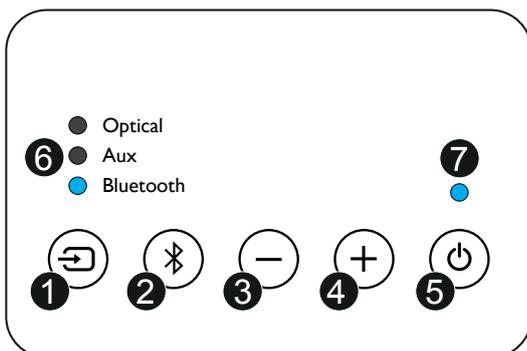
1. Source: Press to cycle through the inputs. This controls what connected device is heard.
