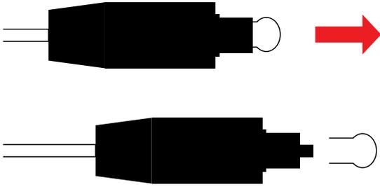
**IMPORTANT:** Remove the protective plastic covers from a new TOSLINK (optical) cable before connecting to the optical sockets. Failure to remove these covers may result in damage and will interrupt the sound output.
