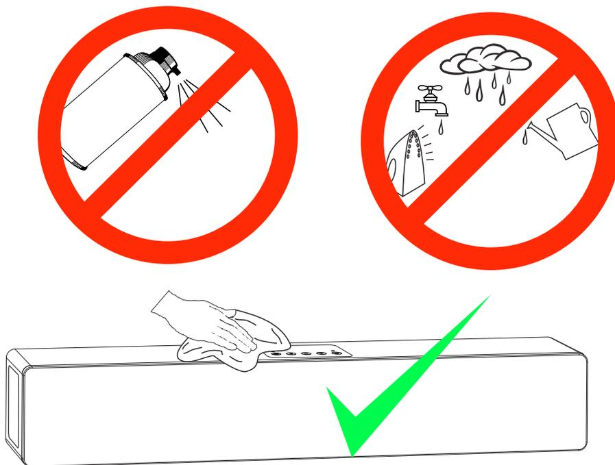
Use a soft, clean cloth moistened with plain, luke-warm water to clean the exterior of the unit. Glass cleaner is a good way to remove finger marks, but please use it sparingly, and avoid contact with the actual loudspeaker driver units.
