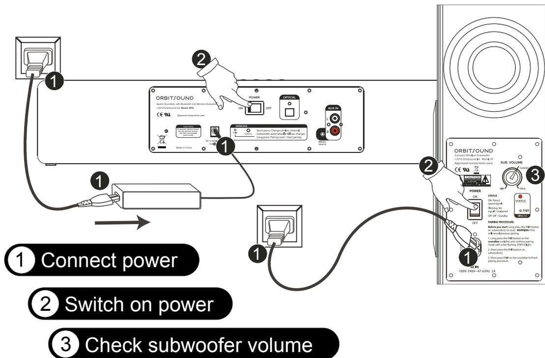
1. Connect the power supply and mains cord to the soundbar. The subwoofer connects directly to the mains via a mains cord (all cables included).
