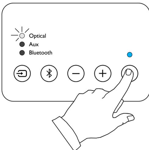
Press the power button. The indicator light will turn blue, and the optical indicator will light, showing the unit is playing the optical source.
