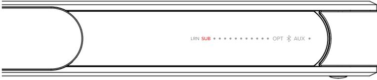
Note: The soundbar shows the red SUB light when there is no subwoofer connected wirelessly. If the subwoofer is on, then it needs to be paired to the soundbar. See 'SUBWOOFER PAIRING'.
