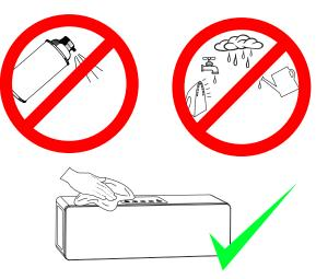
Use a soft, clean cloth moistened with plain, luke-warm water to clean the exterior of the unit. Glass cleaner is a good way to remove finger marks, but please use it sparingly, and avoid contact with the actual loudspeaker driver units.
