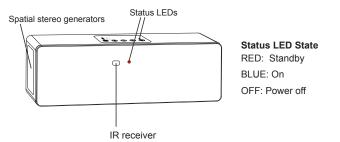
The orbitsound M9LX soundbar produces most of the sound that you hear. It produces the main signal and spatial information.
