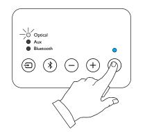
Press the power button. The indicator light will turn blue, and the optical indicator will light, showing the unit is playing the optical source.
