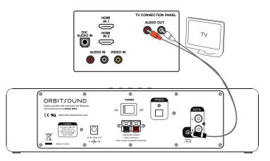
Use the included analogue RCA/Jack cable to connect the audio output from your TV to the soundbar.
