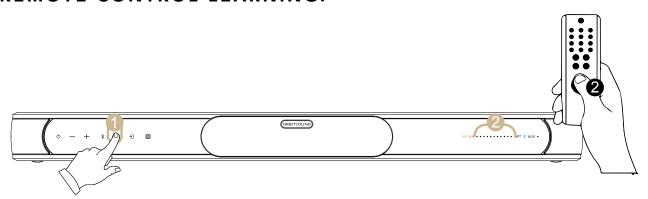
The BAR A70 (and A60) can learn volume control instructions from many other remote control types. The soundbar has the ability to go into a learning mode and to 'scan' a new remote control button, and to use this as a volume control function. This means that when using your BAR, you will not need to reach for the Orbitsound remote in order to adjust the soundbar volume.
