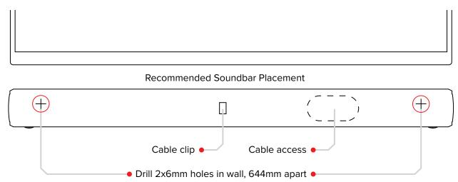
In the package you will find a wall mounting kit. In order to wall mount the soundbar. Wall mounting should only be done by qualified professionals, and the surface for mounting should be sound and strong enough to support the soundbar. If in doubt, install a shelf for the soundbar to sit on.
