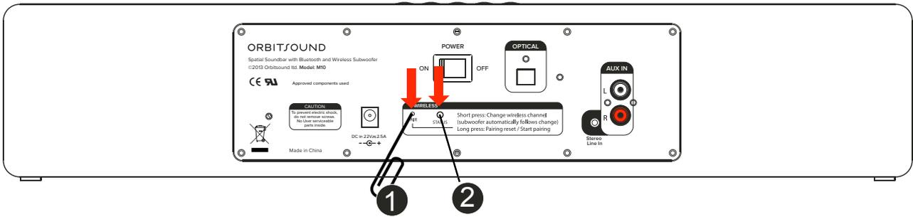
1. Use a paperclip to briefly press the 'PAIR' button on the soundbar rear panel. We recommend changing channel 2 times (2 presses) if you are hearing interference.
